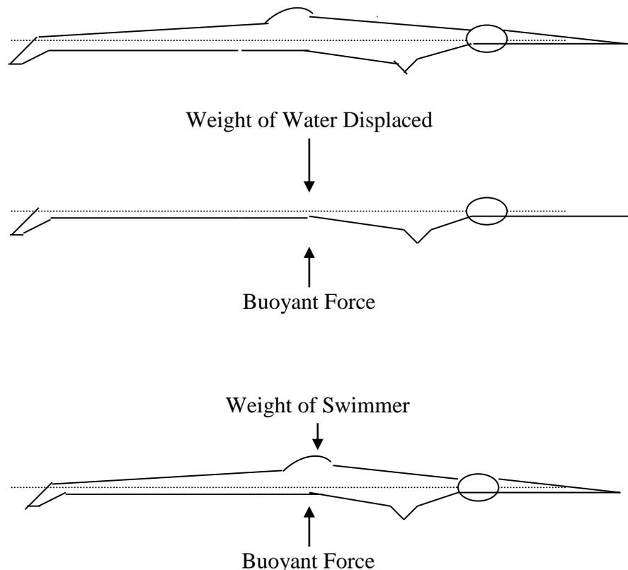
The resultant of this upward vertical force (the so-called buoyant force) that the water exerts must be equal in magnitude to her body weight. This decides whether the body will float or sink. If the weight of the body is more than the buoyant force that the water can provide, the body will sink. If it is not, the body will float. Expressing in mathematical terms, a body will float only if:
