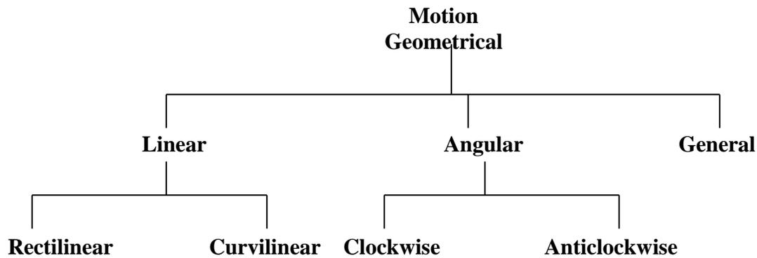
**Linear Motion**-Different parts of the body changes its position in same direction in same time through same distance. Example-Motion of Cg during walking. Running etc.
